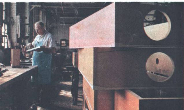
Air to make organ sounds is stored in chambers called reservoirs, shown being built by Omer Vann. There are many old-timers in the business: Vann's been at it 35 years
