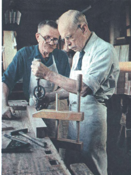
Hector Noterman (r.) drills hole as part of the process of making wooden pipe while carpenter Paulo Fondurko watches
