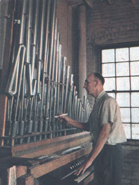
Ralph Bolton of Aeolian-Skinner Co., Boston, tests tone of a set of pipes, called a "stop," on special voicing machine
