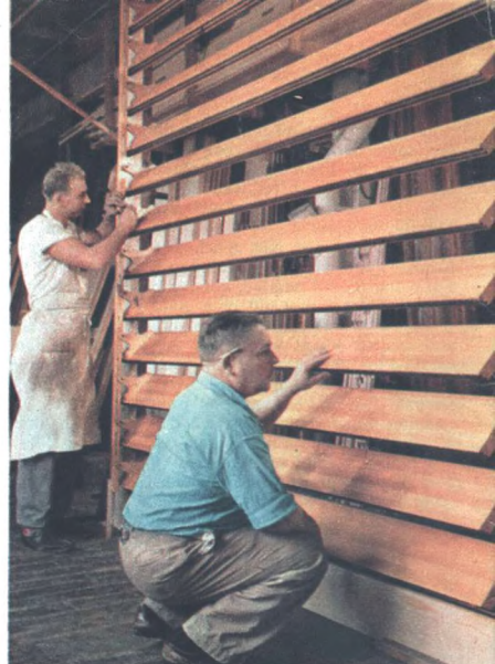
These slats, called "swell shades," regulate the volume of an organ by opening and closing like Venetian blinds
