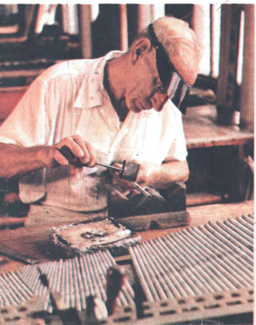
Pipe maker John Robinson soldering a set of pipes, which can be made of metal or other materials. Skilled pipe makers and voicers are profession's top-paid workers
