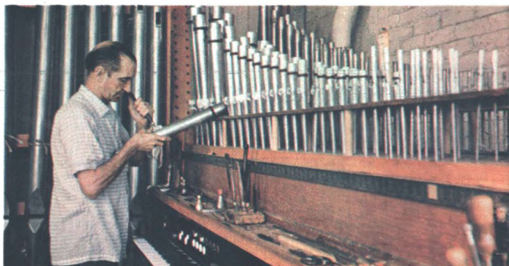
Bill MacKenzie, known as a "flue voicer," checks tonal characteristics of a set of pipes on a voicing machine. Note difference in size between pipes he's testing and those in the background
